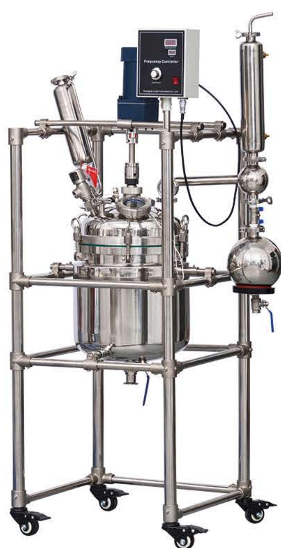
20L stainless steel reactor
