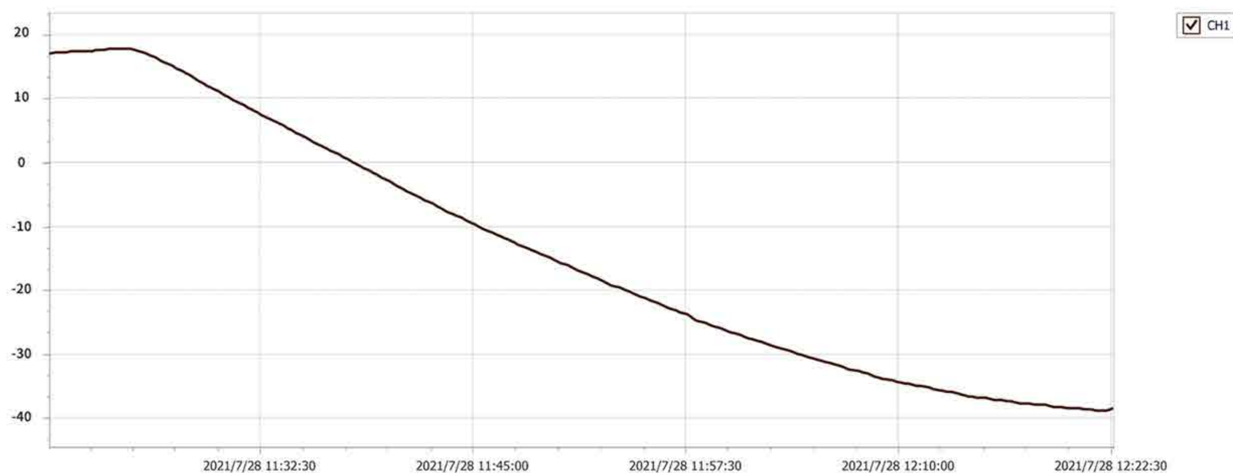
DLSB-50/40 measured temperature control curve in no-load state
